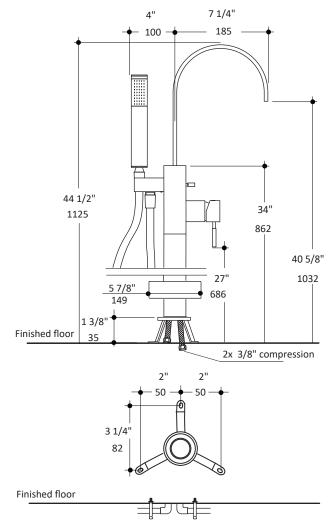
In-floor plumbing connections 2 x 1/2" copper pipe
