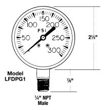
Case and Ring - Black coated steel Bourdon tube copper Socket - Lead Free\* Brass
